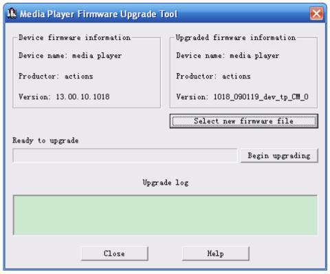
4. Do not disconnect the player from the PC during firmware upgrading or repairing. After the upgrading is completed, a prompt "firmware upgrading succeeded, the program will exit automatically!" pops out. Now confirm, the tool will shut down and reset the player, the whole upgrading is completed.
